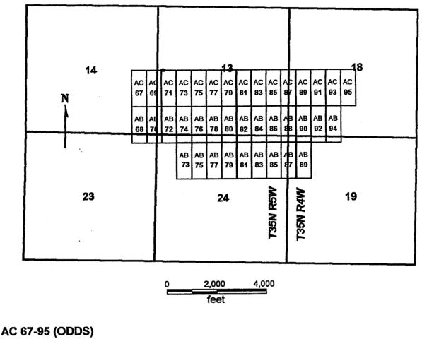
AB 68-94 (EVENS) AB 73-89 (ODDS) Sides are N-S and ends are E-W All locations, corners and end centers are 5' 2x2 wood posts with metal tags
