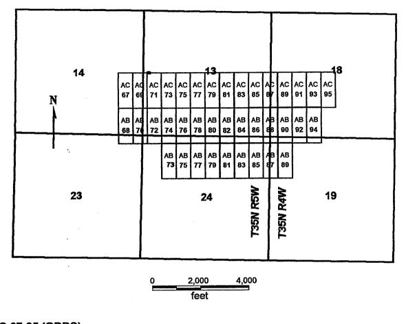
AC 67-95 (ODDS) AB 68-94 (EVENS) AB 73-89 (ODDS) Sides are N-S and ends are E-W All locations, corners and end centers are 5' 2x2 wood posts with metal tags
