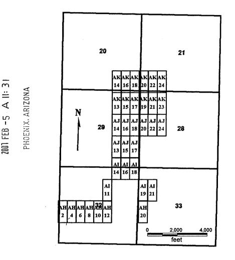
AH 2, 4, 6, 8, 10, 12, 20 AI 11, 14, 16, 18, 19, 21 AJ 13-18, 20, 22, 24 AK 13-24 All claims are 1500 x 600 Sides are N-S and ends are E-W All locations, corners and end centers are 5' 2x2 wood posts with metal tags Located by: Patrick Hillard Mohave Co., Arizona **Box 388**
