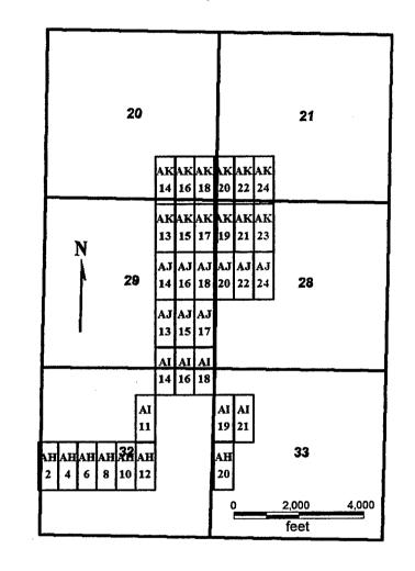
AH 2, 4, 6, 8, 10, 12, 20 AI 11, 14, 16, 18, 19, 21 AJ 13-18, 20, 22, 24 All claims are 1500 x 600 AK 13-24 Sides are N-S and ends are E-W All locations, corners and end centers are 5' 2x2 wood posts with metal tags Located by: Patrick Hillard Mohave Co., Arizona Sections 20, 21, 28, 29, 32, 33 T36N, R5W **Box 388** Gila Salt River Meridian Kanab, Utah 84741
