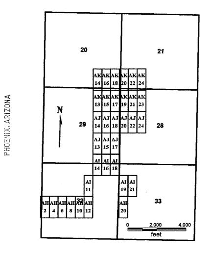
AH 2, 4, 6, 8, 10, 12, 20 AI 11, 14, 16, 18, 19, 21 AJ 13-18, 20, 22, 24 AK 13-24 All claims are 1500 x 600 Sides are N-S and ends are E-W All locations, corners and end centers are 5' 2x2 wood posts with metal tags Located by: Patrick Hillard Mohave Co., Arizona Sections 20, 21, 28, 29, 32, 33 T36N, R5W **Box 388 Gila Salt River Meridian** Kanab, Utah 84741
